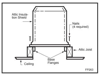
Fig. 20 Attic shield installlation (Canadian requirement).
